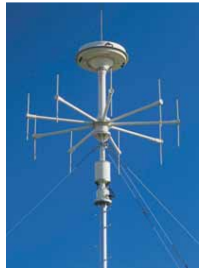
VHF/UHF DF antenna system
